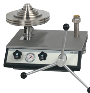
Pneumatic pressure balance, model CPB5000
